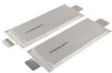
Mixed aged and new cells SOH 90% And aged prismatic cells SOH 80%
